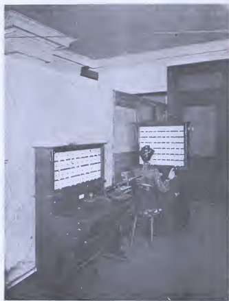
The two Hollerith Electric Tabulating Machines (old model) loaned by the inventor to the Federation.
